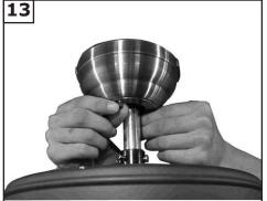
Next lift the canopy disk and install knurled nuts as shown. Tighten the knurled nuts securely. The canopy should adjust for any irregularity in the ceiling or Outlet box.
